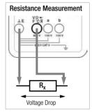
acoustic signal, and "00.00" (+1 digit) appears at the LCD with blinking decimal point. The resistance value measured at the moment the key is pressed serves as a reference value (max. 200 digits). It is automatically subtracted from all subsequent measured values.
